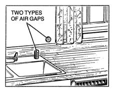
If you have an air gap, check it at least once a month. THE AIR GAP IS NOT PART OF YOUR DISHWASHER. IT IS NOT COVERED IN YOUR WARRANTY. The air gap is easy to clean. With most types, first turn off the dishwasher, then lift off the chrome cover. Then unscrew the plastic cap and check for any build-up of grit. A toothpick makes cleaning easy.
